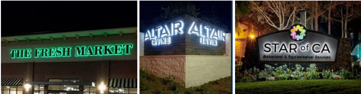
Figure 11- 12. Examples of Backlit Channel Letter Signs
