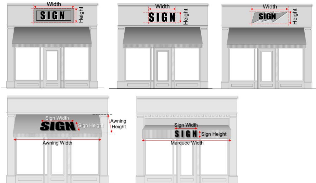
Figure 11- 4. Sign Copy Area Measurement – Building Signs
