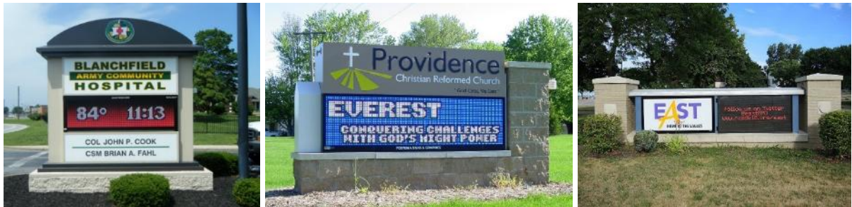
Figure 11- 18. Examples of Changeable Copy Signs
