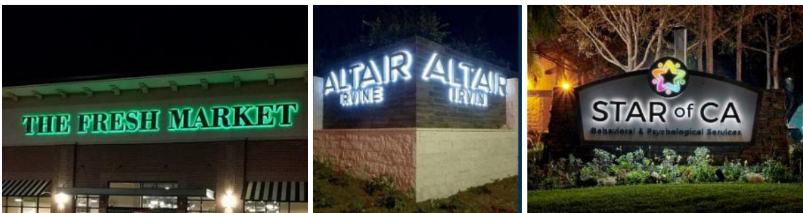
Figure 11- 12. Examples of Backlit Channel Letter Signs
