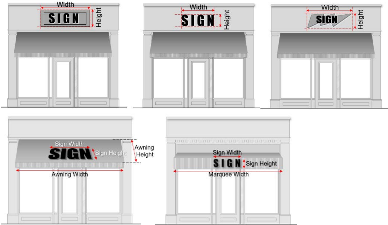
Figure 11- 4. Sign Copy Area Measurement – Building Signs
