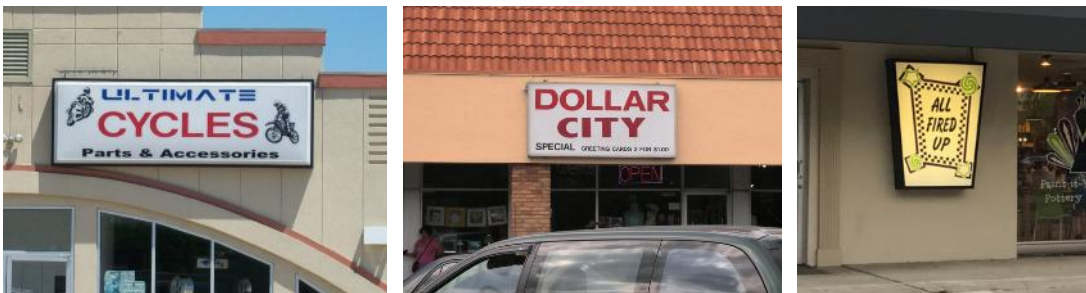
Figure 11- 10. Examples of Prohibited Cabinet Sign Illumination
