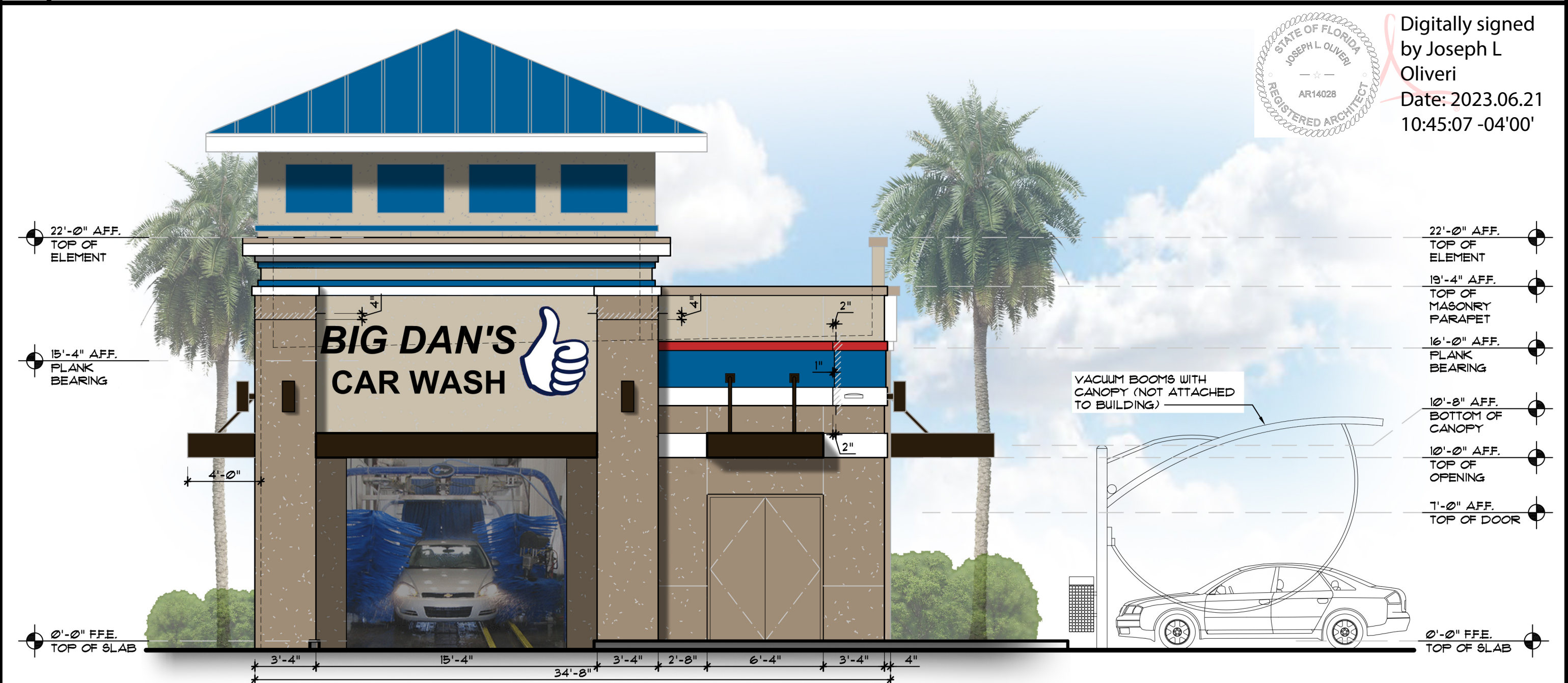
3 NORTH EXTERIOR ELEVATION - TUNNEL EXIT SCALE: 3/16" = 1'-0"
