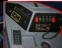
Authentic working pump control valve, rocker switch panels, communication hardware, and gear shift panel
