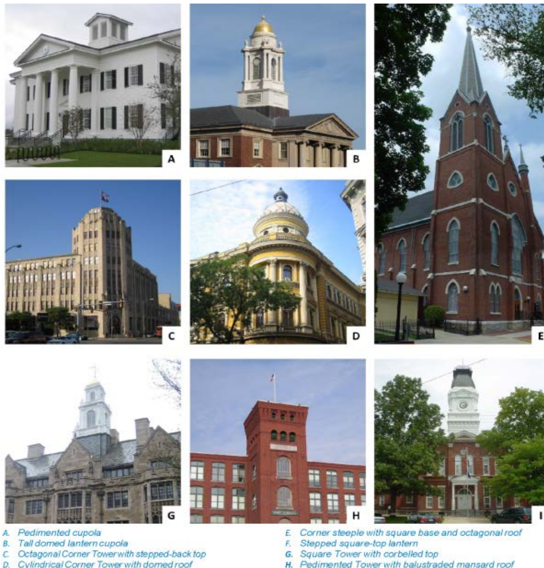
Figure 5-31. Examples of Small Footprint Towers/Cupolas
