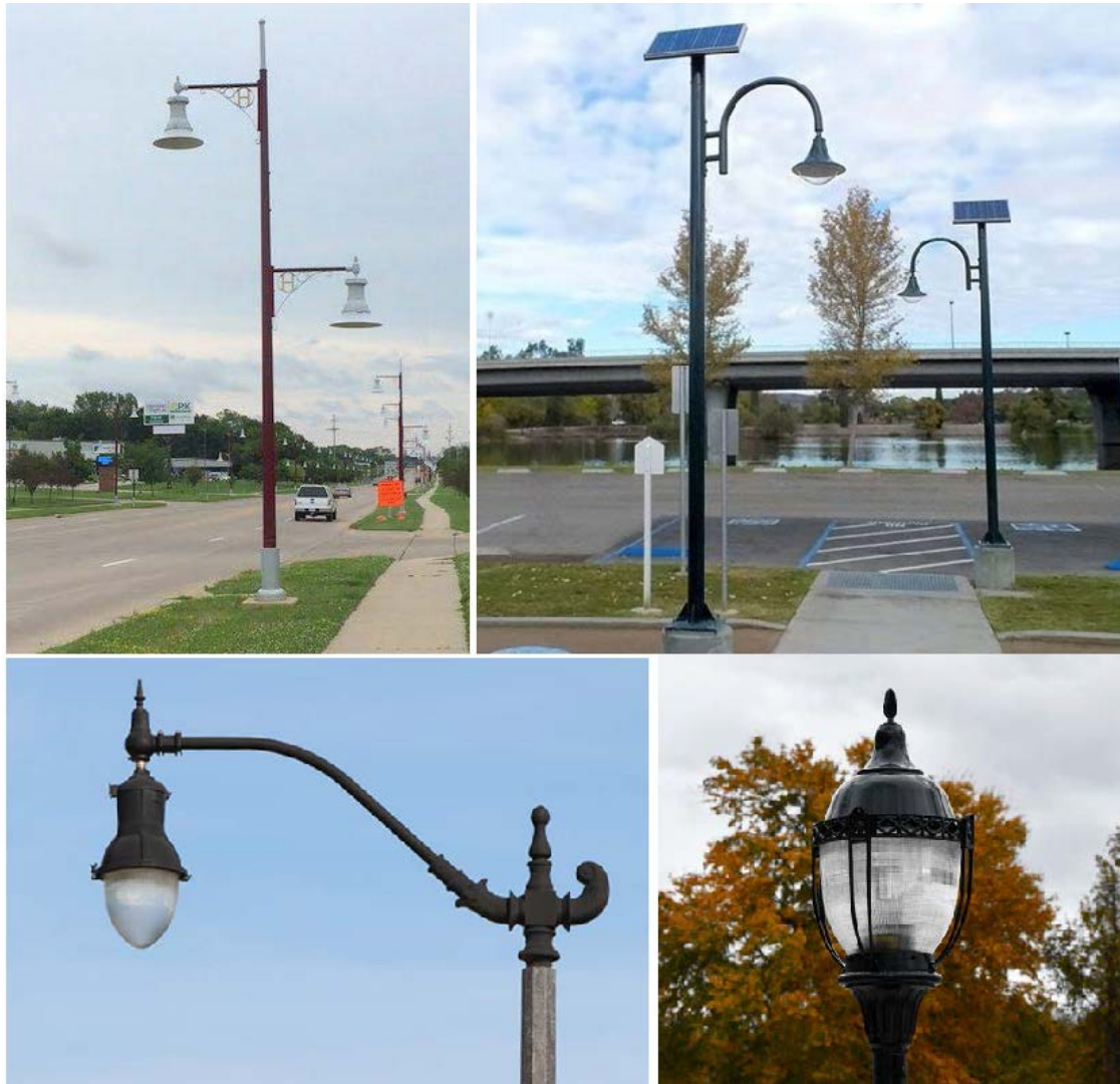
Figure 7-1: Examples of Streetlight Fixtures
