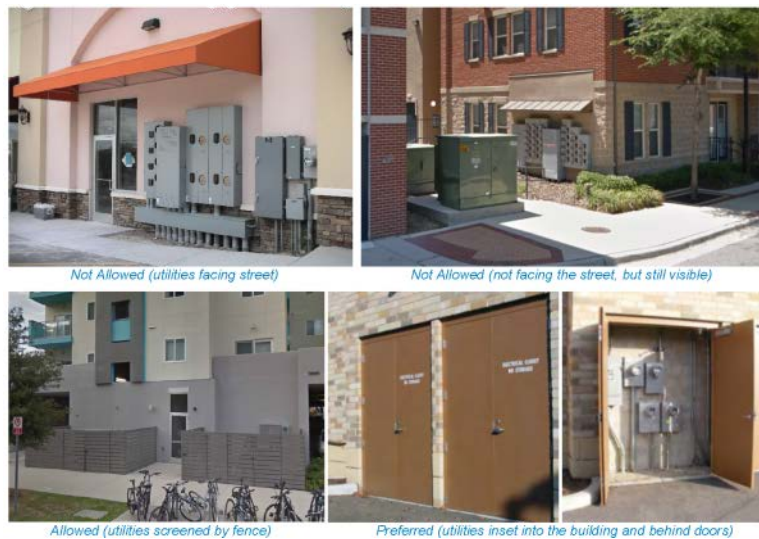
Figure 5-46: Mechanical Equipment Screening
