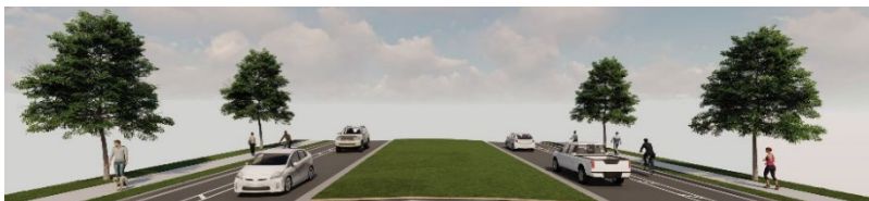
Figure 1: Hybrid Typical Section (initial 2-lane)
